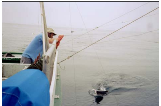
Figure 77: Having used his hydraulic salmon gurdies to bring the fish to the surface, commercial fisherman Tom Stickel must now hand pull the last 15-18 feet of monofilament in order to land a Chinook salmon. Photo by Barbara Stickel.
