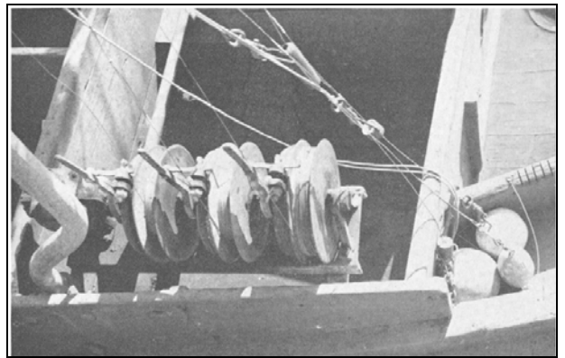
Figure 76: Three salmon gurdies mounted on a single shaft. There is a second set of three on the other side of the boat. The lines are stainless steel. Note the three lead weights at the right. Photo by D. H. Fry, Jr., 1949 (Fry 1949:42).
